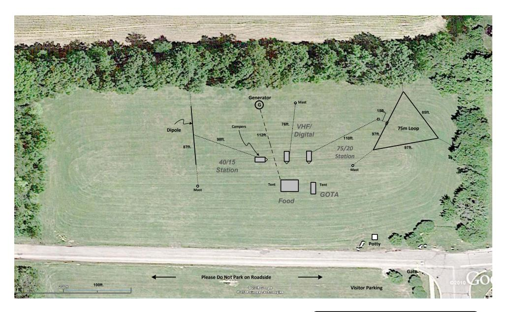
Location: 3711 S Casper Drive, New Berlin Lat. 42.976828; Lon. -88.119637 Field is approx 600 ft E - W; 250 ft N - S Elevation: 943 ft at East end; 920 ft at West end Drawing scale: 1 in. = 70 ft.
