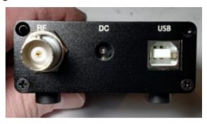
The QDX operates on the 20/30/40/80 meter bands at approximately 5W output and can be powered by a 9V or 12V battery, your choice. It has a built in sound card, USB serial COM port, internal VFO and is completely controlled via CAT commands from your attached computer. Literally, by plugging a laptop into the USB port and an antenna into the BNC, you've got a complete, ready to go digital station.
