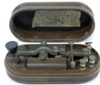
This miniature portable key was easily carried in a pocket. used by telegraph linesmen to test lines back to their depot. Circa 1850.
