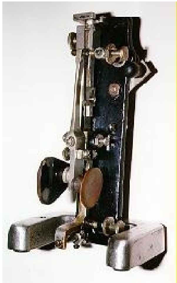
6265 VIBROPLEX VERTICAL "LINE CHIEF'S KEY:(10KB) Labeled: Trade VIBROPLEX Mark, No. 63440 U.S.Patents 767,303, 812,183, 842,154, 1,042,457, 1,043,449, 1,074,831, 1,109,818, 1,110,373, 1,170,796 1,178,291. THE VIBROPLEX COMPANY INC. 253 Broadway, New York.Circa 1918.
