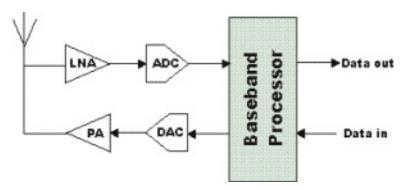
Tier 3: The ideal software radio or ISR where the boundary between configurable and non-configurable elements exists very close to the antenna, and the "front end" is configurable. It could be said to have full programmability.
