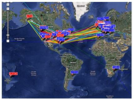
Database: A list of WSPR activity being reported. Database query parameters may be set to limit results to a specific band, transmitting station, reporting station, etc.
