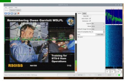
Turns out the RPi does a great job of encoding and decoding SSTV. I used my Pi at Field Day for the FT8 digital station and SSTV is just another digital mode to the Pi. Keep in mind, my Pi is a RPi-2, so it is ancient tech in the RPi world. I downloaded the QSSTV package and was literally up and running in 15 minutes. Once setup, it runs and catalogs the pictures automatically. It ran all weekend without a hiccup. That's pretty cool.
