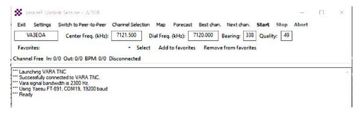
The recommended procedure at this point is to click on the Channel Selection button at the top of the window. This will open the Channel Selector Window which you should then update by clicking on the Update Via Internet button and then Exit.
