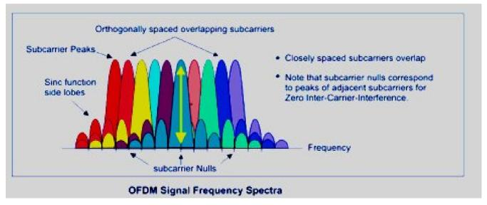
VARA uses OFDM modulation which, to grossly oversimplify, allows parallel information transfer via multiple subcarriers in a single transmission channel. The speed increase results from transmitting the information simultaneously via the multiple paths. The long and short: it can be blazingly fast. But then we run into the pesky FCC mandated Symbol Rate limitation. I'm not going there in this discussion, but be aware of the restrictions for use within the US
