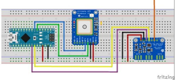
This is how I wired up the breakout boards into the simple WSPR beacon. Connect your laptop to the Arduino Nano. This not only powers your transmitter but lets you download the program from the Arduino development program.
