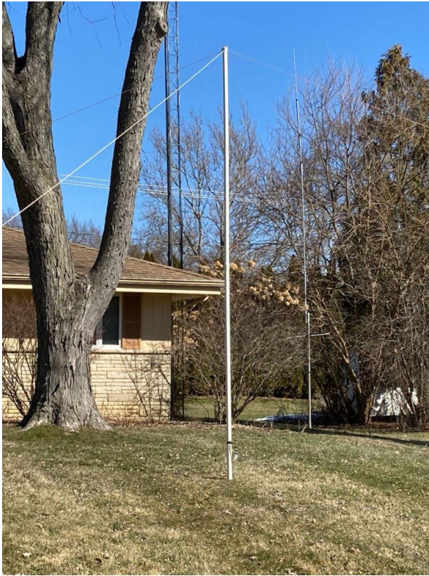
NVIS design by N6VNG (sk) from 1998. SWR less than 3:1 across most of 1-30 MHz.
